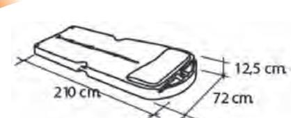
WEIGHT 14 kg - MATERIAL: POLYETHYLENE
