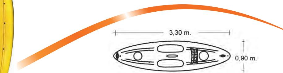
WEIGHT 22 kg - MATERIAL: POLYETHYLENE
