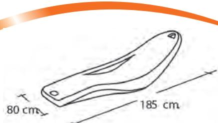
WEIGHT 14 kg - MATERIAL: POLYETHYLENE
