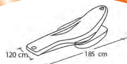
WEIGHT 18 kg - MATERIAL: POLYETHYLENE
